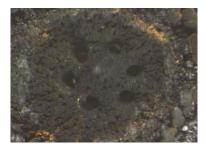
GDI fuel injector nozzle tip with coked deposits, <u>after 48 hr Dirty-Up</u> (DU) test phase.
