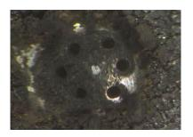
GDI fuel injector nozzle tip with coked deposits, <u>after 24 hr Clean-Up</u> (CU) test phase.
