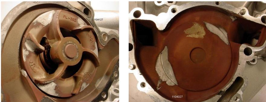
Mind you, scales and deposits only 1/16" thick can reduce heat transfer by up to 40%! The longer coolant gel is allowed to recirculate through a cooling system, the more time it has to completely drop out of solution and form scales and deposits. This will eventually result in overheating.
